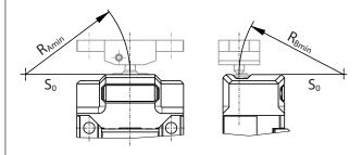
$R_{\text{Amin}}$  and  $R_{\text{Bmin}}$  depend on the actuator. Applies accordingly also to lateral retraction directions.
